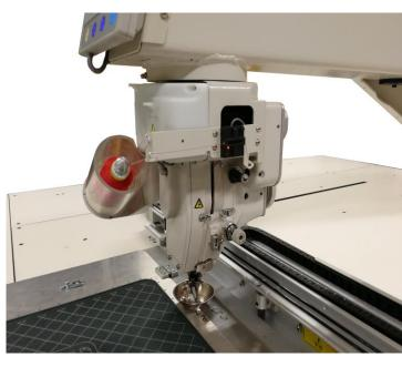
The special 360° rotating head has been designed to guarantee the same stitch quality in every direction. Is particularly proper for 0 tolerance on irregular stitches productions. The rotating block has a spool holder and a thread breakage sensor. The machine is provided with a special window on the working table that allows to the operator to replace the bobbin easily and quickly.
