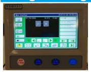
Touch programmable panel, easy and intuitive. It allows to the operator to choose with program to run and modify it immediately.
