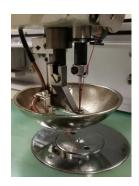
Special presser foot, adjustable in height and pressure directly from the touch panel, it guarantees a uniform pressure even on multilayered materials.
